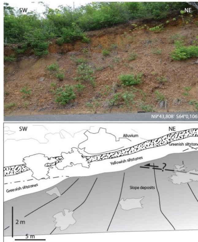
Figure 3.18. Reverse surface faulting associated with the Tarragona thrust. Outcrop photo (top) and its interpretation (bottom). The contact between yellowish and greenish siltstones shows a gently north-dipping reverse fault that tilted the upper alluvium layer.
