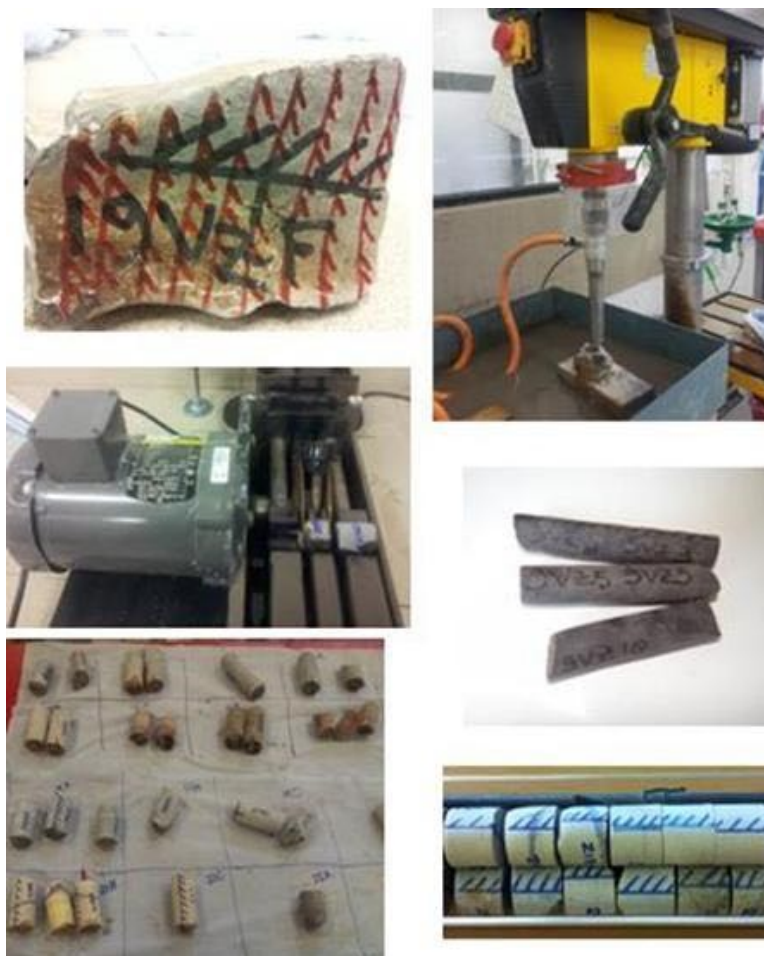
Figure 5.29. Drilling, cutting and preparation of the oriented blocks in the laboratory at the University of Burgos, Spain.
