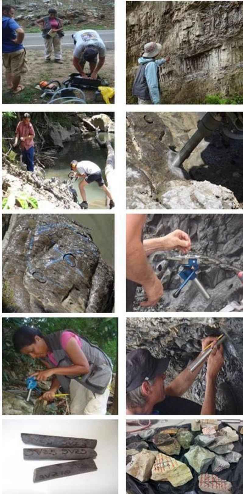
Figure 5.24. Drilling, orientation in-situ and sample acquisition in the field.
